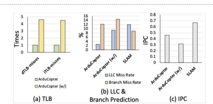
(a) ArduCopter with SLAM dTLBand iTLB misses normalized to only execute ArduCopter. (b) LLC and branch prediction miss rates for ArduCopter, ArduCopter with SLAM, and SLAM.(c) IPC for ArduCopter, ArduCopter with SLAM, and SLAM.
