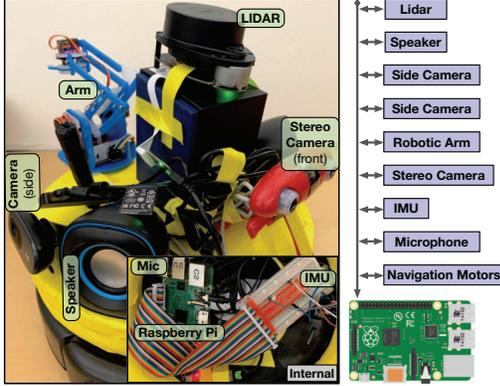
Fig. 1: Modified iRobot with RPi4 and additional sensors.
